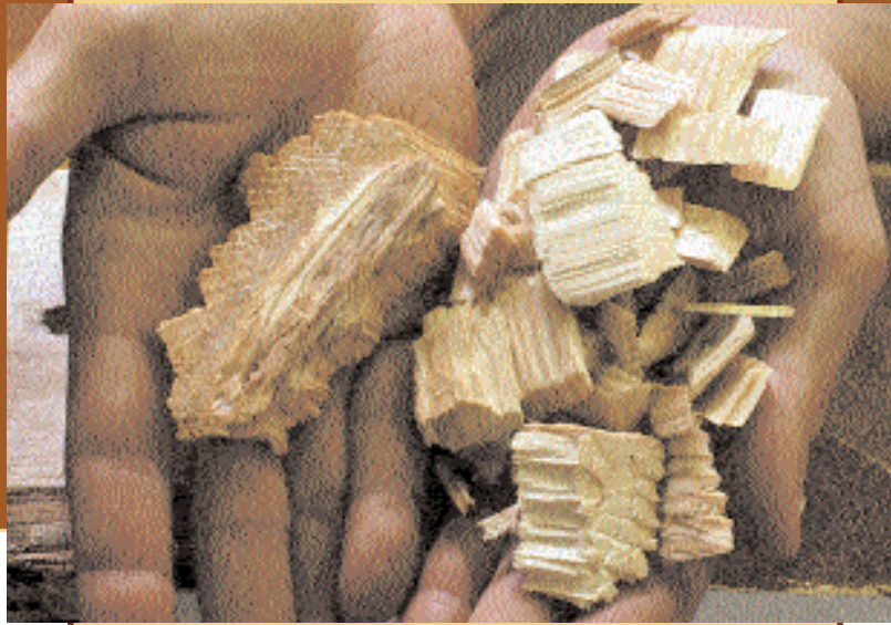
The wood chip on the left has been treated with fungus, making it easier to break down in the pulping process. The chips on the right have not been treated, and will require more chemicals or a longer treatment when they are pulped.
